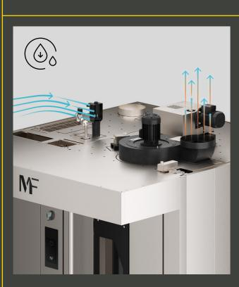
Speed Dry ensures greater crunchiness and shelf life for each product. Its use reduces the time needed to evacuate steam into the chamber by 70%.
