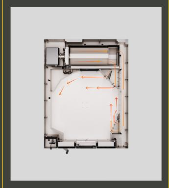
The DAF (Double Air Flow) system allows for maximum cooking uniformity even with intensive or short cooking times. The entry of hot air into the chamber from two directions allows for a more homogeneous distribution of heat.
